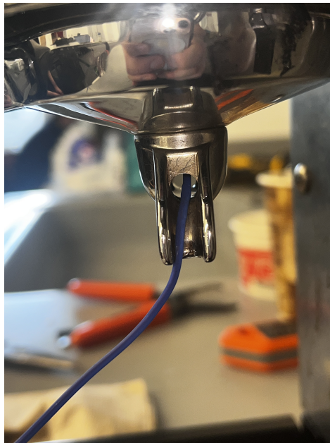
Fig. 7 Brewing Water Thermocouple Placement
